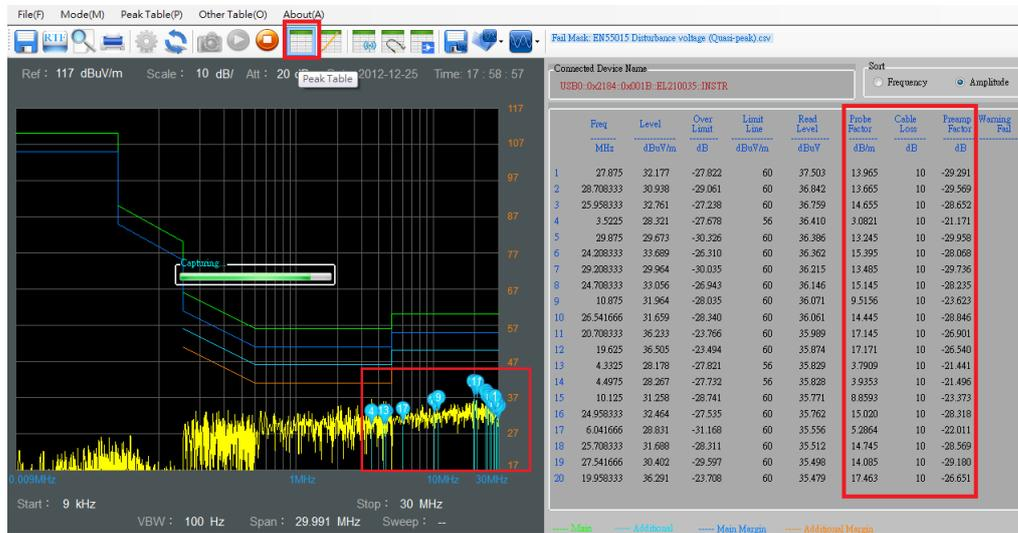
When some frequency points exceed the Fail/Warning Mask, "Warning" or "Fail" will be displayed on the screen.
