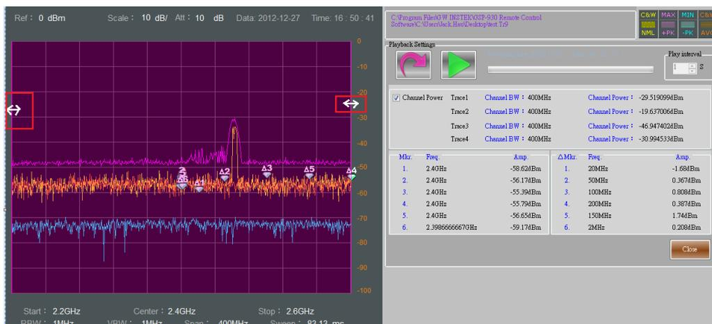
For example, below the 'Channel BW' was set to '40MHz' to measure the 'Channel Power' of 'Trace 1~4'.
