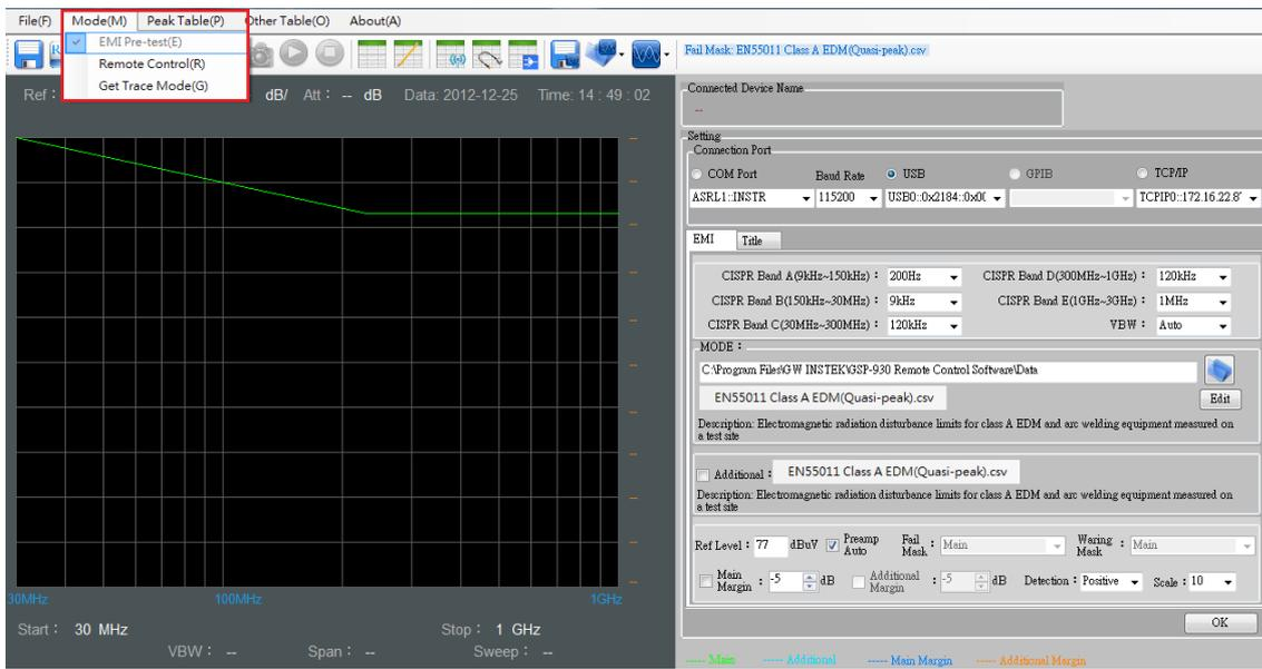
You can select the required CISPR EMI regulation, including conduction and radiation measurement within SpectrumShot.
