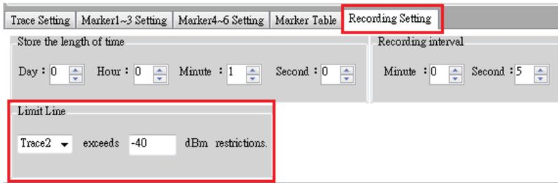
Please fill in the form below before ticking the 'Open the send mail function' check box. When the measurement triggering conditions and Limit Lines have been set up, SpectrumShot will automatically send an email to you. There are two ways of sending an email: 'Single' and 'Repeat'. 'Repeat' sending means that you can set a fixed time interval between each email (e.g. every 10 minutes).
