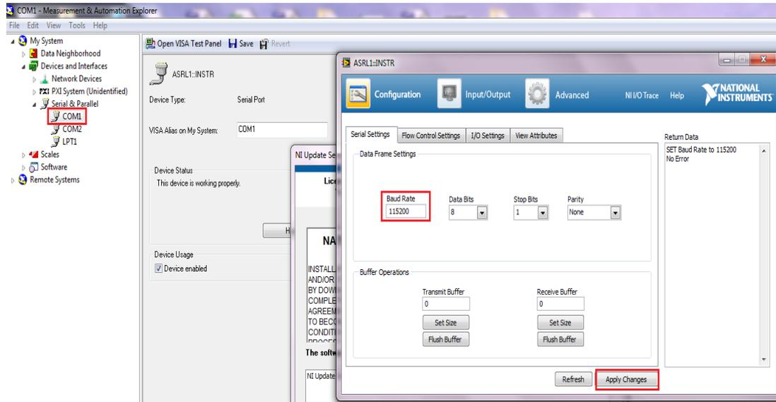
To check that data can be read from the spectrum analyzer, you can go to the NI 488.2 Input/Output setting and execute the `*IDN?` command.
