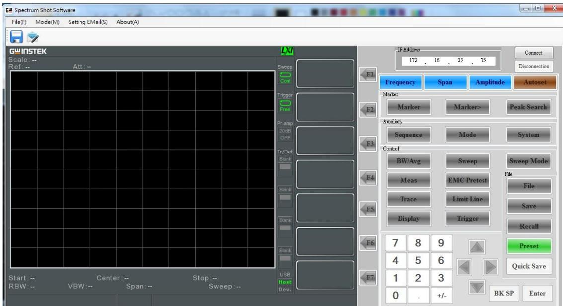
Before connecting, you can set up the 'Setting Email' function. When the general account and message information is filled out, tick "Open the send email function" check box. When the test results match the original setting condition, SpectrumShot will automatically send an email to the address specified.
