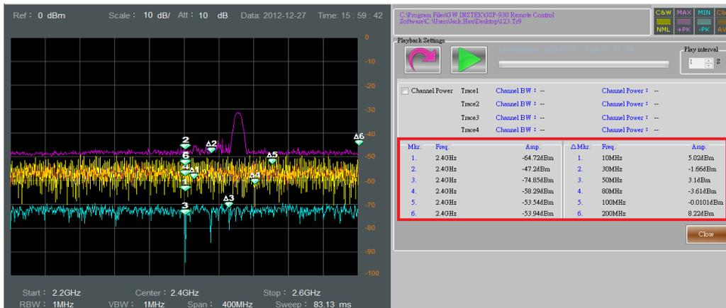
If you want to acquire the 'Channel Power' within the test result, they can tick 'Channel Power' check box. The program will then display a purple background to indicate the bandwidth. You can use the mouse on the purple background to redefine the bandwidth.
