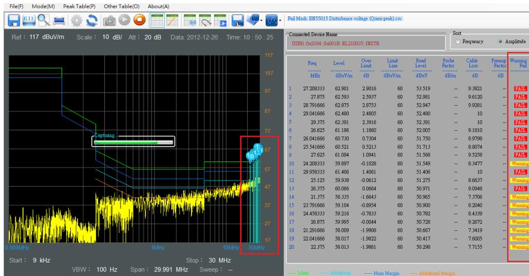
The peak points can be user-defined with the Edit Peak Table function. You can directly click the SpectrumShot test result with a mouse or fill-in the frequency column. Refer to the graph demonstrated below.
