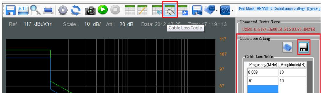
The Gain value should be set below zero when you connect the Spectrum Analyzer with external pre-amplifier.
