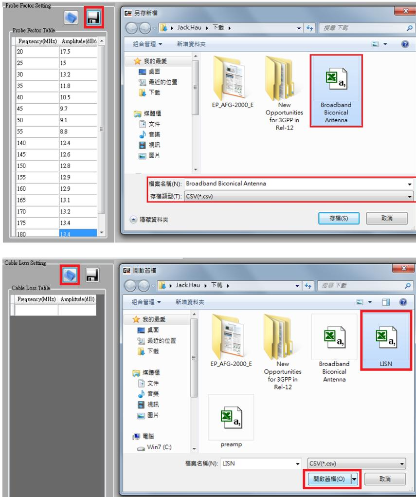
You can search the frequency and amplitude of the 'Warning or Fail' masks under the Peak Table option. Here, the the Probe factor, Cable loss or Preamp factor may also be shown on the diagram. The Peak Table option will search for 20 peak points in the test result.
