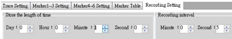
After setting up the recording time, select the 'Recording' button, then save as \*.Tr9 format.
