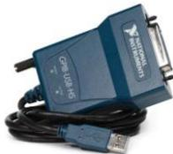
If you need to use the NI GPIB to USB Adaptor (GWINSTEK GTL-251), then the NI-488.2 driver should be installed in advance.
