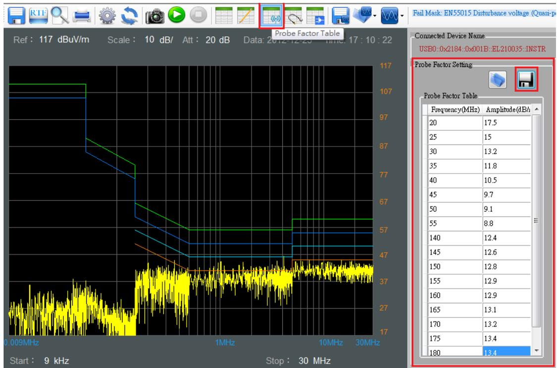
If you know the insertion loss of the cable, LISN, or pulse limiter, it can be inserted and stored in this column.
