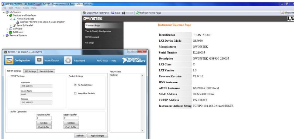
To check that data can be read from the spectrum analyzer, you can go to the NI 488.2 Input/Output setting and execute the \*IDN?\n command.
