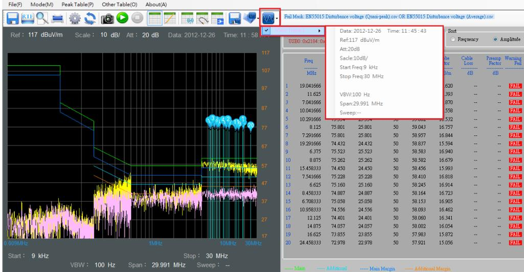
If you want to store the test result of a DUT in a text file, you can press the ‘Save to rtf’ button. The tables will then be saved in the rich text file format (\*.rtf). An informative description of DUT can be entered and saved under the “Title” tab.
