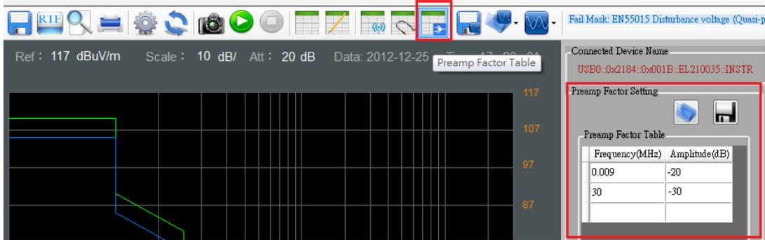
The Probe, cable loss and Pre-amp settings are saved in a \*.csv format, which can be opened and edited by Microsoft Excel.
