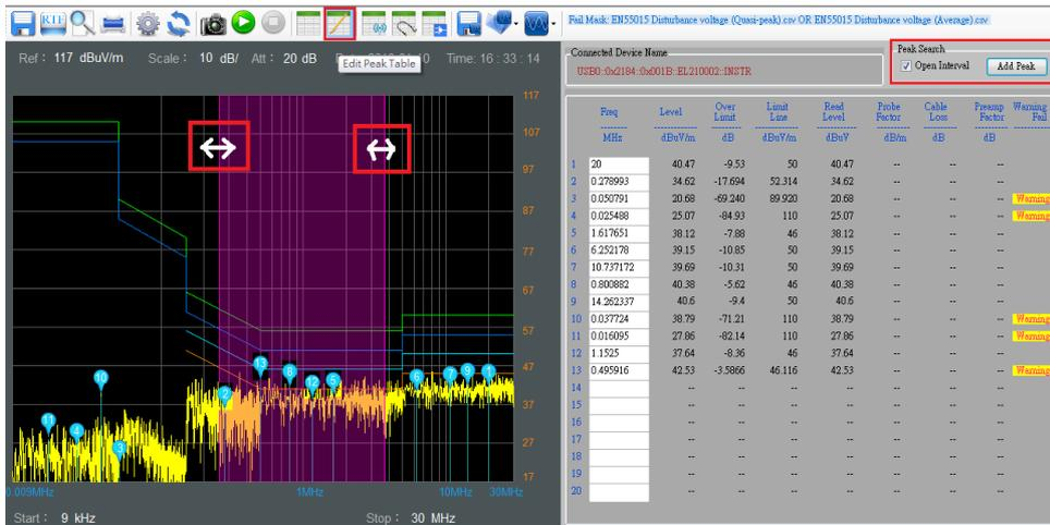
If you need to compare the test results from different DUTs, the test result can be saved as \*.CSV file format.
